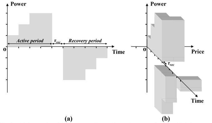
Fig. 2. (a) Example of the processed set-point trajectory  $s(k+i|k)$  which is sent at time instant  $k=0$ . (b) Three dimensional plot of the processed set-point trajectory  $s(k+i|k)$  accompanied with prices. In both figures time is discretised in  $i$  steps, while the x-axis represents the control horizon.
