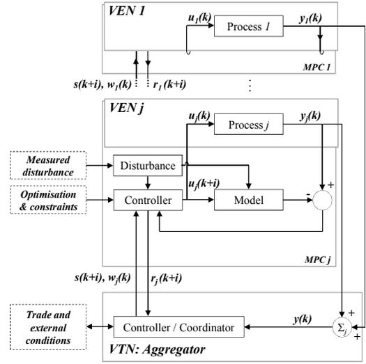
Fig. 3. Illustration of the real-time operations at time instant  $k$ . The VTN represents the aggregator that has a number of associated VEN, while the  $j$ -th VEN is illustrated together with the MPC block.
